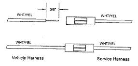
4. Stretch both harnesses so the wires lay side-byside. Select a vehicle harness wire, locate the matching color on the service harness. Cut the vehicle harness wire at the midpoint of the butt splice.
