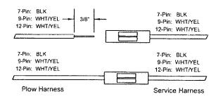
Stretch both harnesses so the wires lay side-byside. Select a plow harness wire, locate the matching color on the service harness. Cut the plow harness wire at the midpoint of the butt splice.
